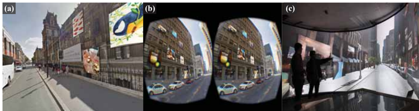
Figure 1: Results from our system, Social Street View. (a) shows the rendering results in a regular display. Users can look through the museum in Paris for geo-tagged artworks inside as well as the dishes in nearby restaurants. (b) shows the stereo rendering results in a VR headset. Geo-tagged images are automatically aligned with building geometry and laid out aesthetically. (c) shows the deployment in an immersive curved screen environment with 15 projectors. Users can explore hundreds of social media messages near a New York city street at a resolution of 6k \times 3k pixels. Please refer to the supplementary video at http://augmentarium.umd.edu and http://socialstreetview.com .
