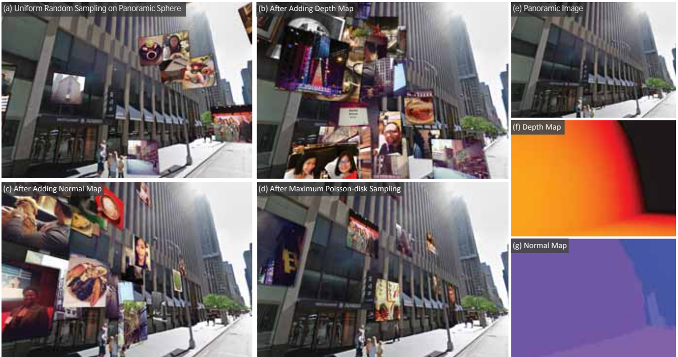
Figure 5: Results before and after applying the depth map, the normal map and maximal Poisson-disk sampling. (a) shows the random layouts generated uniformly on the sphere, (b) shows results after using the depth map, (c) shows results after applying the normal map, (d) show results after using maximal Poisson-disk distribution for laying out photographs, (e) shows the original street view image, (f) and (g) visualize the depth map and the normal map respectively, for reference
