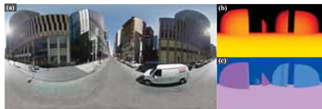
Figure 3: The illustration of (a) stitched panoramic image tiles, (b) depth map and (c) normal map from Google Street View. The depth map is visualized in a yellow-red-black color scheme, where black indicates 255 meters or more, red indicates 128 meters and yellow indicates 0 meters. The normal map contains a 3D normal vector for each pixel. We visualize the normal data by converting the normal vector to HSV color space with blue-purple hues.
